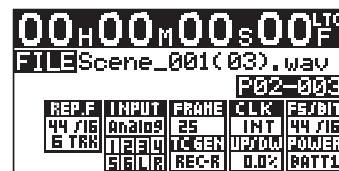
A Home screen example when the ES Device ID is set to "03"
